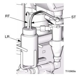
FIG. 10. Pump Lubrication System
