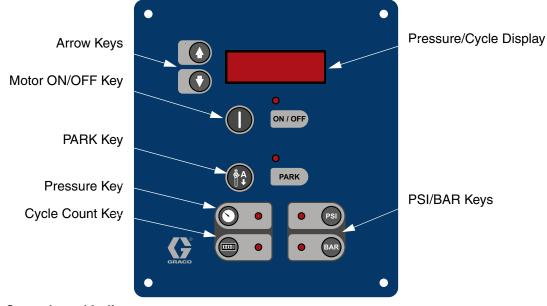
FIG. 5. Motor Controls and Indicators
