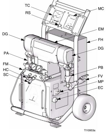
FIG. 3: Component Identification (Model EXP-1 Shown)
